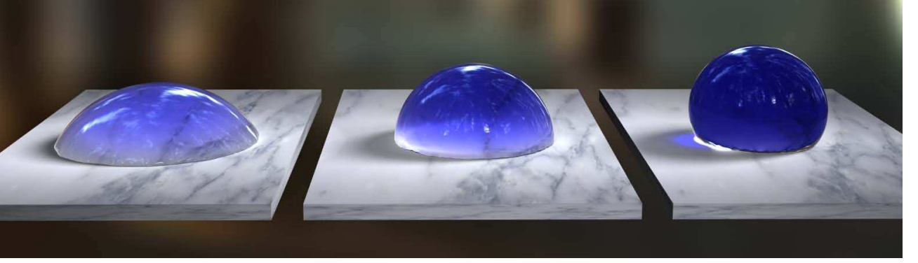
Fig. 2: Droplets on the solid surfaces with different contact angles. They are 60, 90, and 120 degrees form left to right.
